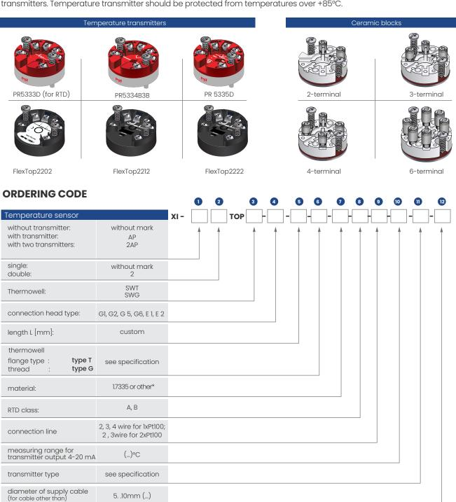
**EXAMPLE** Temperature sensor XI-TOPSWG-G1-500-1/2NPT-1.4541-A-3 **3 4 5 6 7 8**
