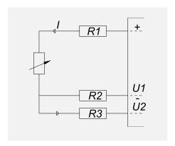
Interconnect wires must have the same resistance R1=R2=R3. The following table gives an example of errors in 3-wire connection for Pt100 and Pt1000 for the difference in wire resistance  $0.1\Omega$  and  $1\Omega$ .
